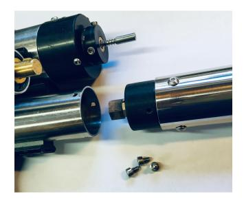
Extension Lance easily connects directly to the rear section of the ZE7000 Pin Brazing Gun to bypass the trigger.
